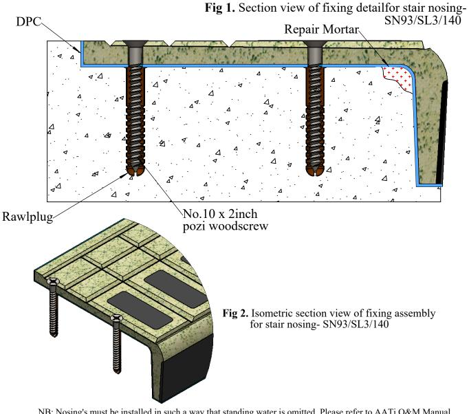
NB: Nosing's must be installed in such a way that standing water is omitted. Please refer to AATi O&M Manual All AATi products are subject to our manufacturing tolerances and should be taken into consideration when installing
