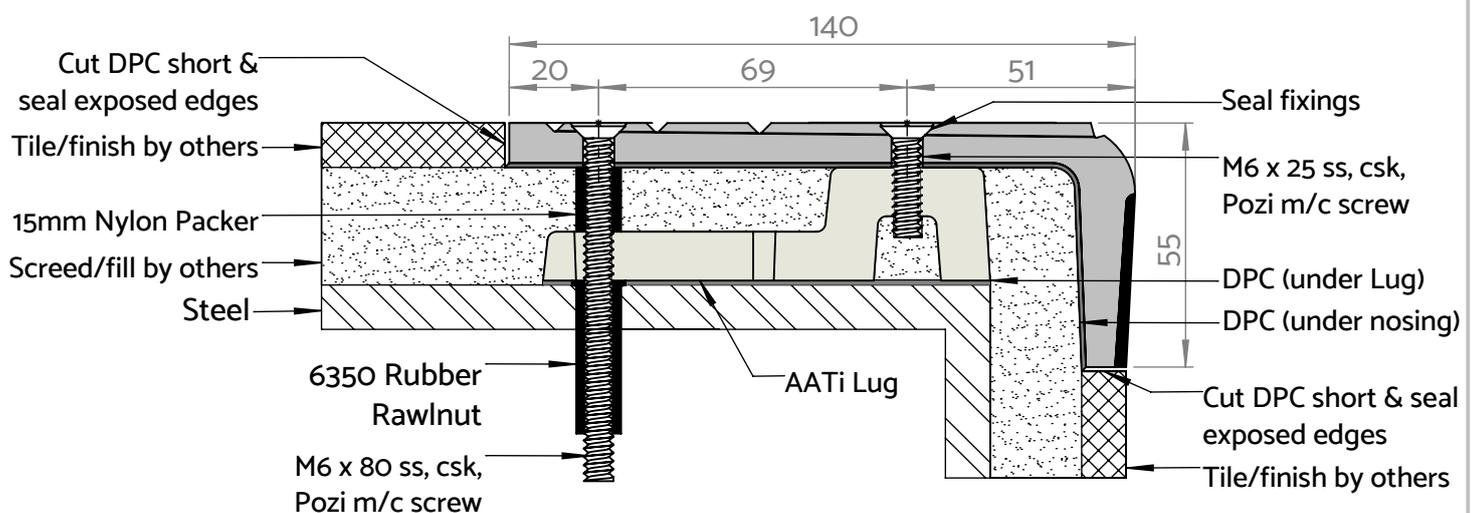
NB: Nosing's must be installed in such a way that standing water is omitted. Please refer to AATi O&M Manual
